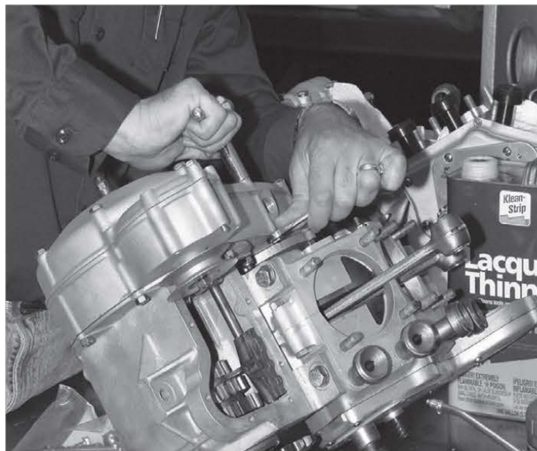
Primary drive with Kiwi anti chatter clutch
